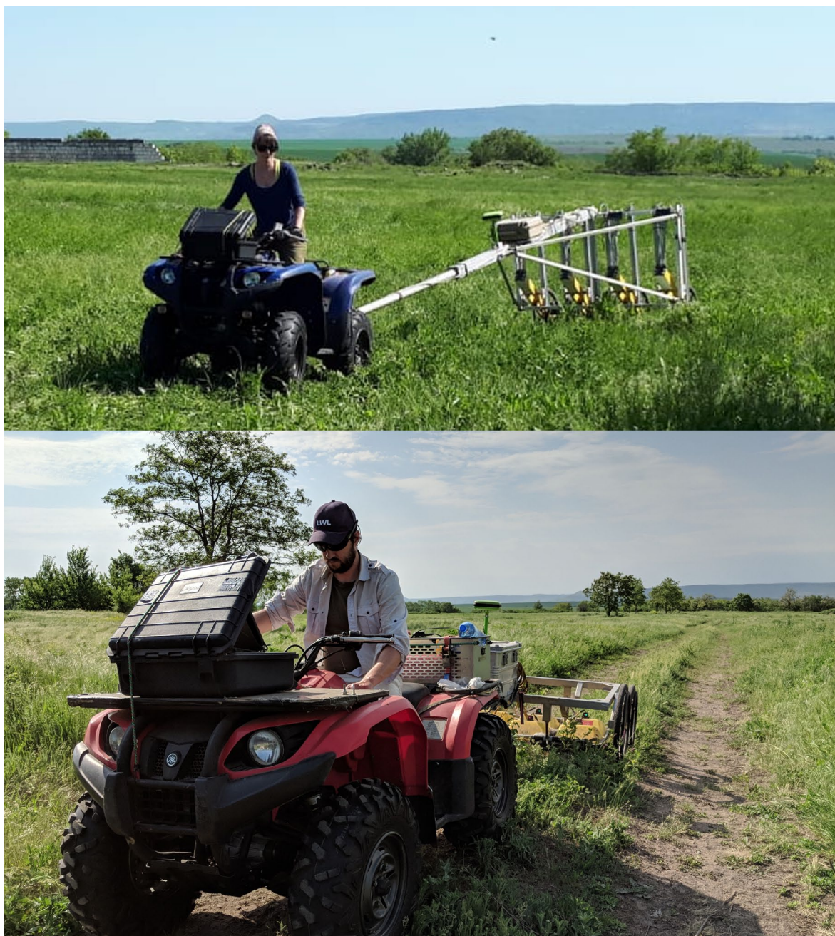
Fig. 4. Survey systems applied at Pliska in 2018: A fluxgate magnetometer system (above) and a 250 MHz GPR-system (below) (photos by M. Gamon and J. Schlegel)
