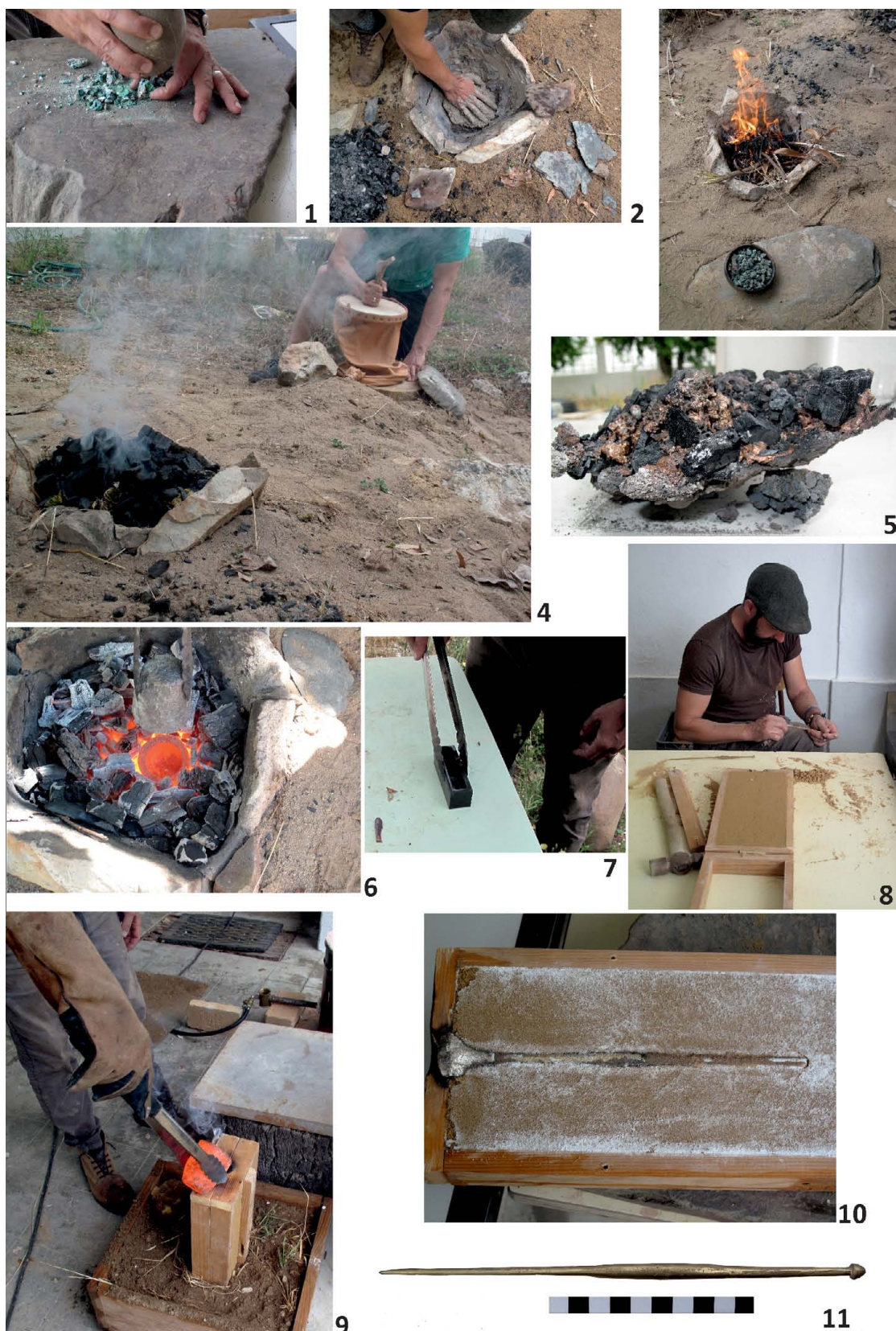
Fig. 1. Experimental reconstruction of manufacture of a Thracian type bronze fibula from the copper smelting process to the obtaining of a semi-finished object (photos M. Stamberova)
