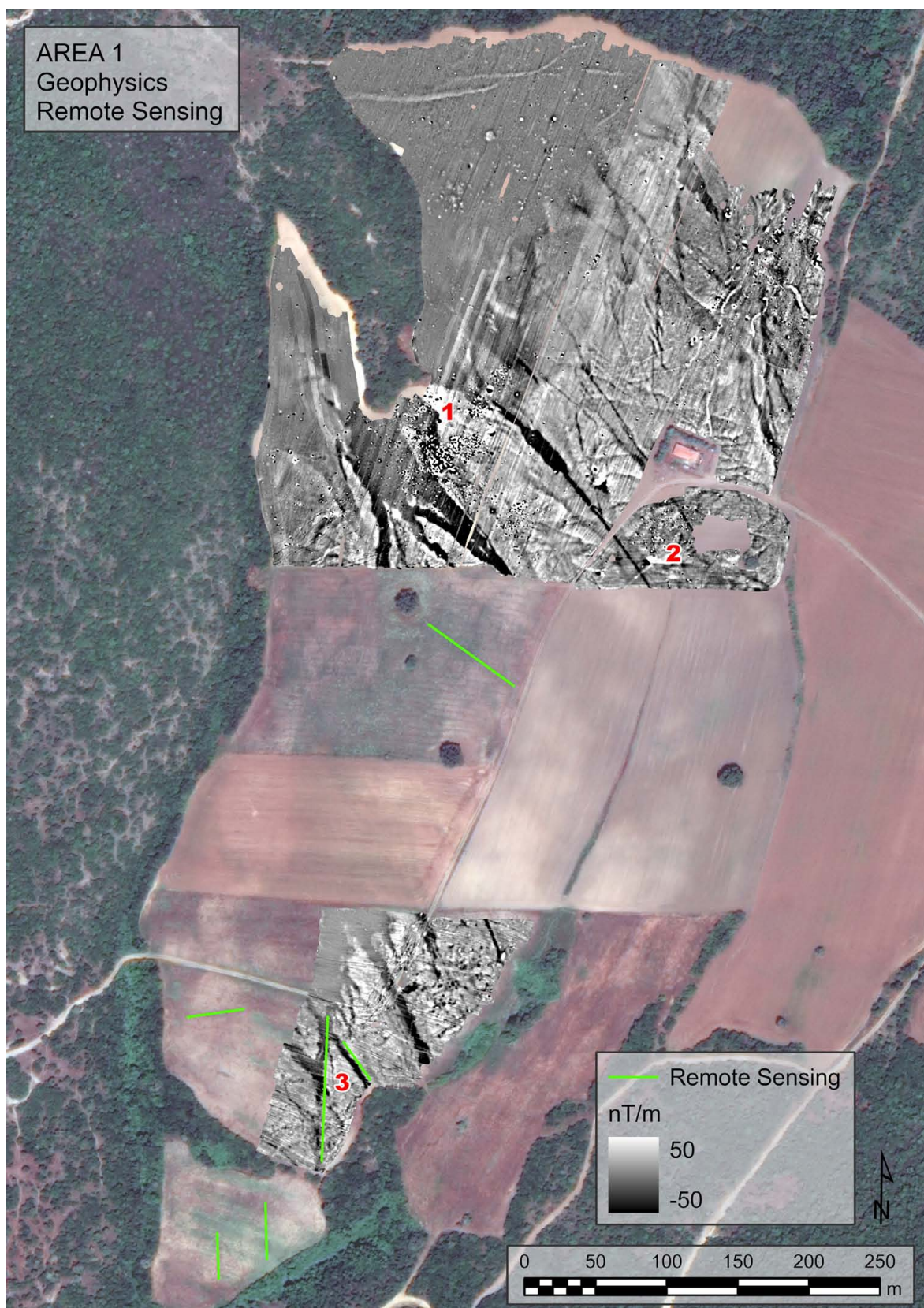
Fig. 9. Results of magnetics survey and satellite remote sensing from Area 1 (figure by J.C. Donati and N. Papadopoulos)
