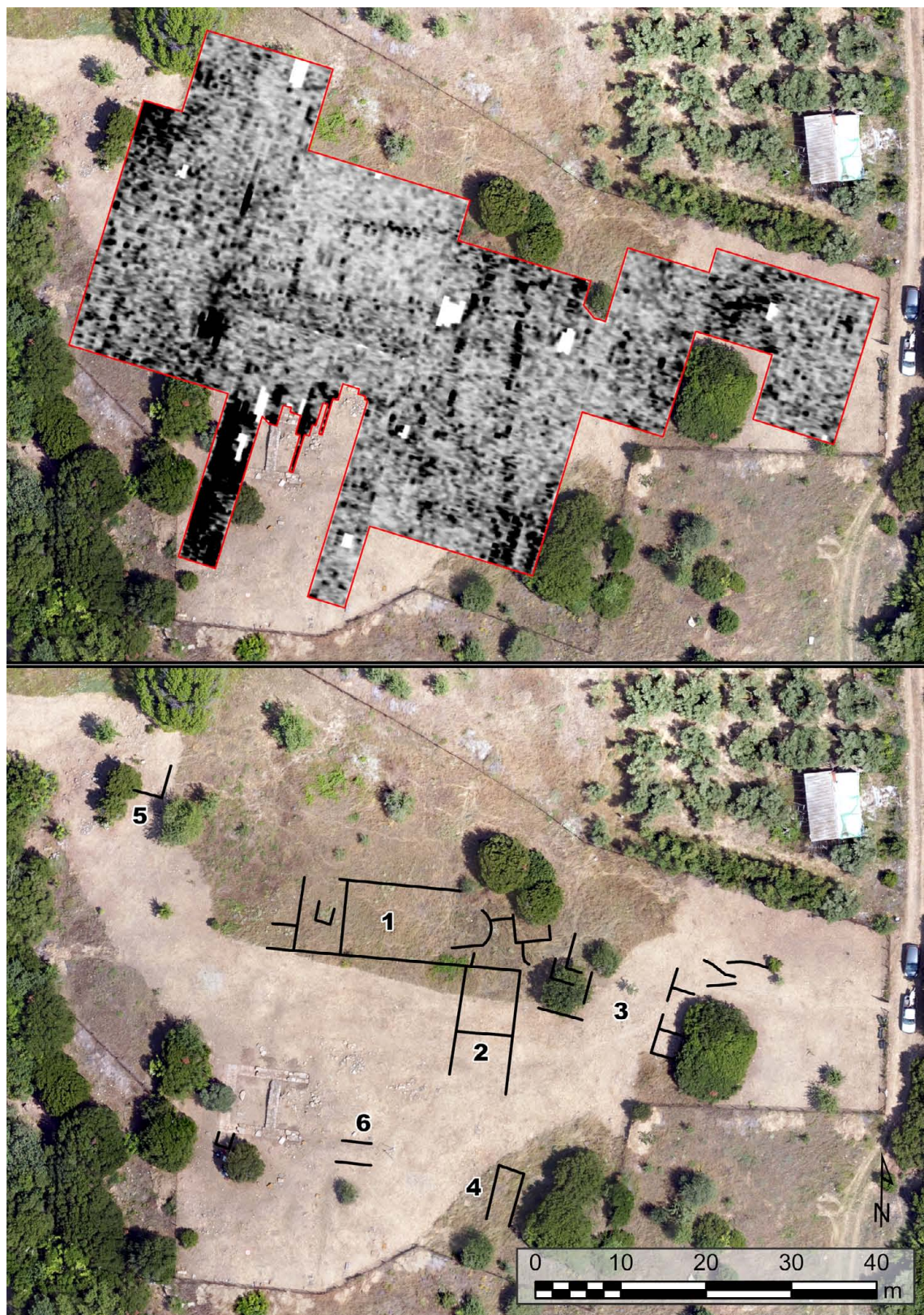
Fig. 13. Results of GPR survey (depth slice 0.80–0.90 m) on plateau of Area 2 (top); interpretation of the results showing possible buried architecture (bottom) (figure by J.C. Donati and N. Papadopoulos)
